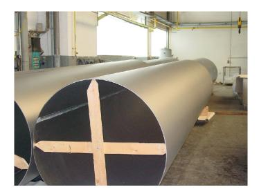
Tubes formed from sheet and welded, 100% x-ray, pickled, for refinery/for chimney
