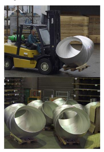
Segment elbows formed from sheet and welded, 100%x-ray, pickled, for refinery/for chimney
